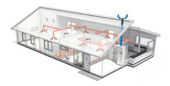
Exhaust air with preheated supply air
