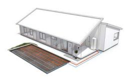
Surface soil – using a surface collector
