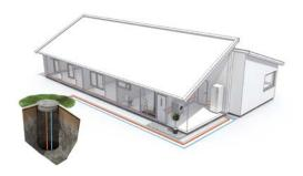
Rock - using a ground probe
