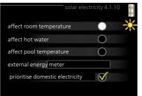
This is where you set which part of your installation (room temperature, hot water temperature, pool temperature) is to benefit from the solar electricity surplus.
