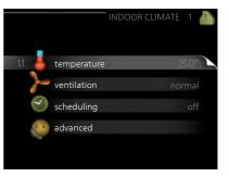
ventilation Setting the fan speed. The status information shows the selected setting. This menu is only displayed if the exhaust air module is connected (accessory).
