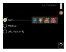
The control module operating mode is usually set to "auto". It is also possible to set the control module to "add. heat only", when only additional heat is used, or "manual" and then select what functions are to be permitted.
