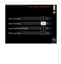
When the operating mode is set to "auto", the control module selects when start and stop of additional heat and heat production is permitted, depending on the average outdoor temperature. If the heat pump has the integrated cooling function and it is activated in the menu you can also select the start temperature for cooling.
