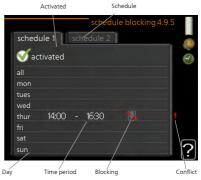
*Day:* Select which day or days of the week the scheduling is to apply to here. To remove the scheduling for a particular day, the time for that day must be reset by setting the start time to the same as the stop time. If the row "all" is used, all days in the period are set according to that row.
