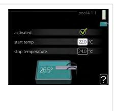
Select whether the pool control is to be activated, within what temperatures (start and stop temperature) pool heating must occur and how many compressors may work against the pool at the same time.
