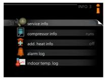
compressor info shows operating times, number of starts etc for the compressor in the heat pump.
