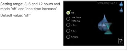
When hot water requirement has temporarily increased this menu can be used to select an increase in the hot water temperature to lux mode for a selectable time.
